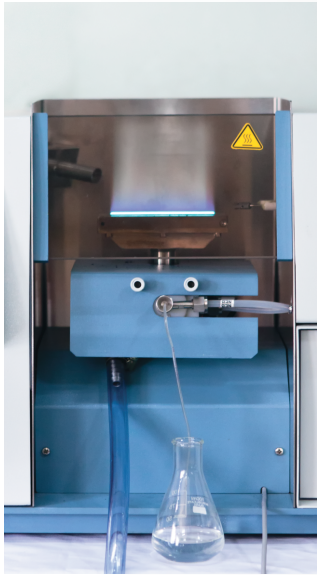
Auto Burner Assembly with Air - Acetylene Flame
