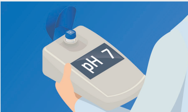
5. Mix the necessary reagent with the water sample, Insert the sample in the instrument and START the Sample analysis.
